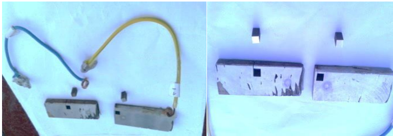
Figure 4 Samples preparation for electrochemical test
