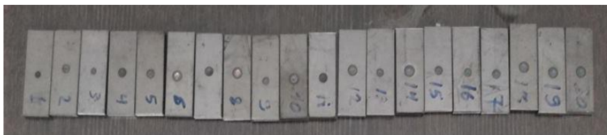
Figure 3. Some samples after welding process.
